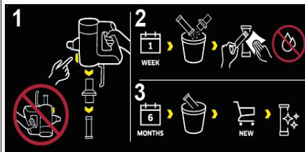
There is a sticker on the pre-filter of the device that describes the cleaning / replacement of the pre- and fine filter.
